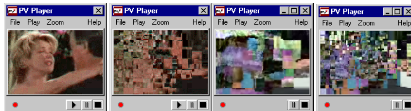
Figure 1: Example sequence (from Left to Right): Original, Encrypt VLC only, Encrypt FLC, and Encrypt VLC&FLC.
