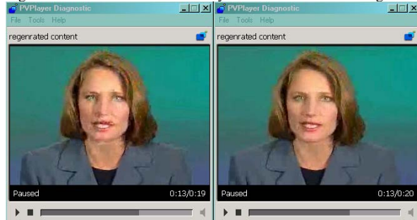
Fig. 5: Reconstructed frames at the same timestamp (at about 13s) after switching. Left: simple switching scheme based on client request; Right: proposed R-D optimized switching scheme.
