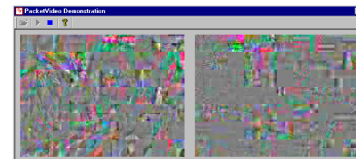
Fig. 2: Attacked frame of Fig. 1 by setting DC of luminance component to 128, DC of chrominance components to 0, and all MV to 0.
